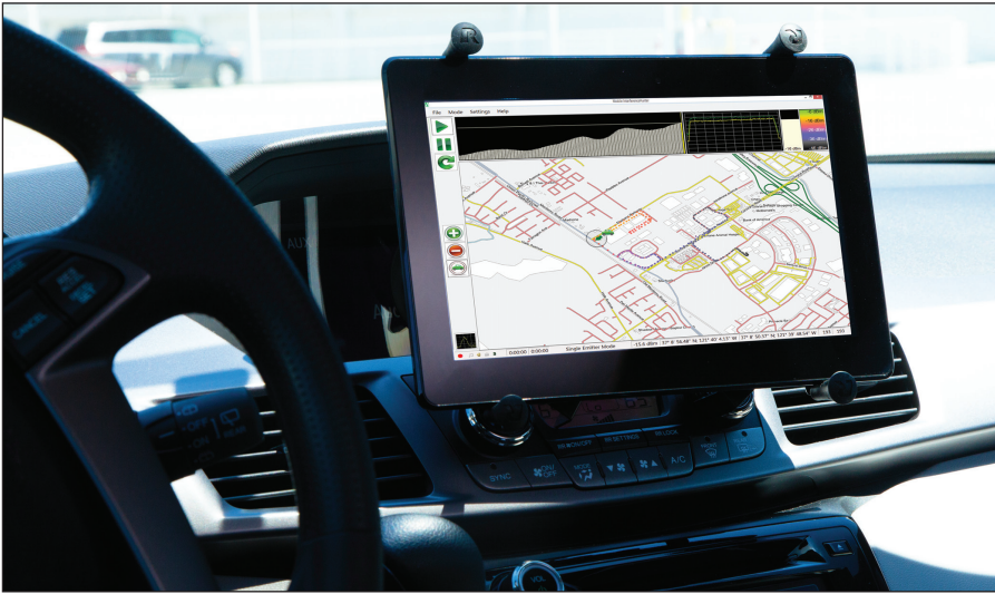
Mobile InterferenceHunter™ on Windows® PC Tablet with Spectrum Master™ in Vehicle
